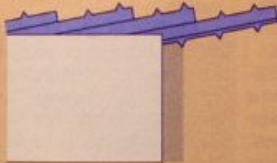
(b) Jet grouting "umbrella arches"
