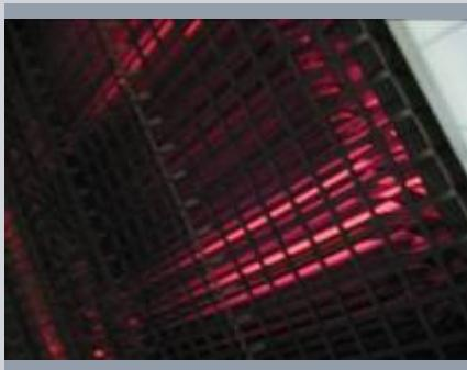
Static test of the safe electric brake in Dresden
