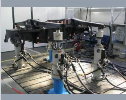
Static and dynamic tests of the bogie frame in Graz Plant
